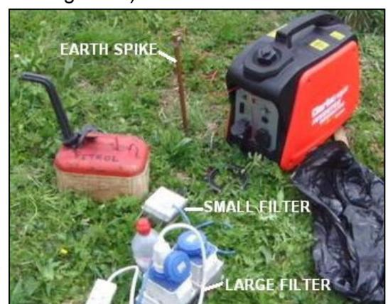
Figure 1- Typical Setup
